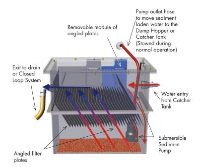
**Water Filtration Process**: Red/blue arrows indicate a slow moving, laminar water flow ideal for the maximum settling of small and lightweight particles
