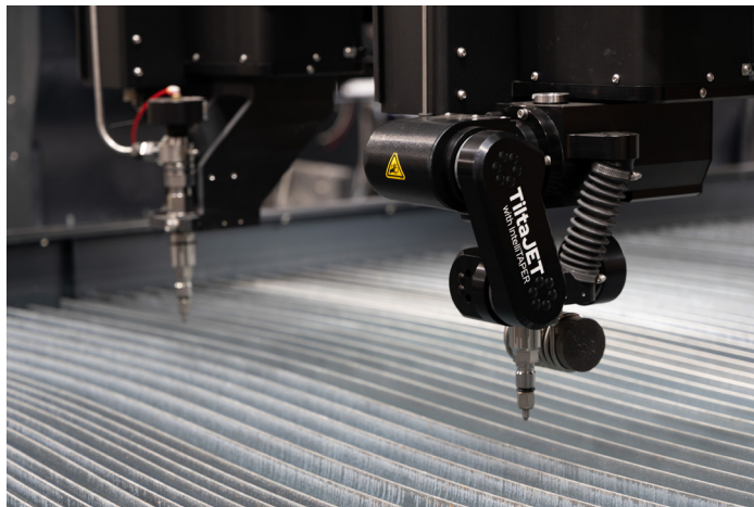
Control both carriages on the OptiMAX Dual Carriage from a single mobile controller, reducing footprint and simplifying operator workload.
