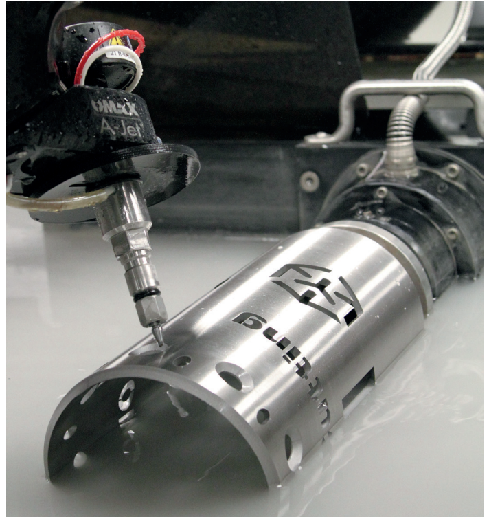
When used with the A-Jet, fishmouth intersections, saddle cuts, and countersunk holes can be cut along the circumference of pipes.
