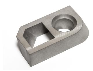
The VersaJET helps eliminate tapers and makes cutting bevels simple.
